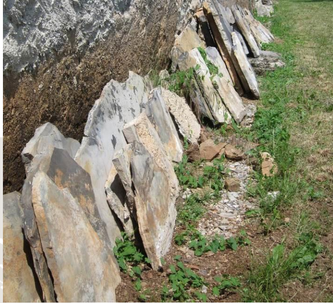
Figure 5.3 Limestone slabs of Komen platy limestone from the Povir Fm. ready for use.
