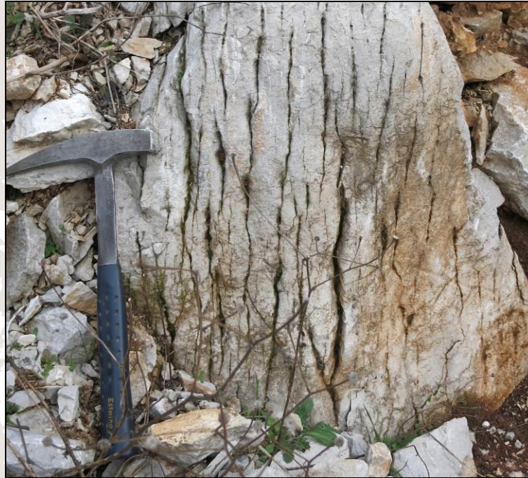
Figure 3.10 Fractured Repen limestone in the Griža (Tavčar) quarry near Povir. The dense system of parallel vertical tectonic fissures enable the excavation of thin limestone plates. They were widely used for roofing in the nearby villages of Divača, Gorenje and Povir.
