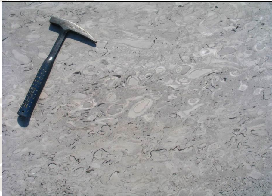
Figure 2.3 The structure of Repen limestone type (easily visible mainly un-fragmented rudist shells)
