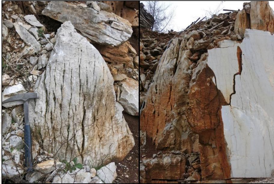
Figure 4.23 Fractured Repen limestone in Griža (Tavčar) quarry near Povir. The dense system of parallel vertical tectonic fissures enable excavating thin limestone plates.
