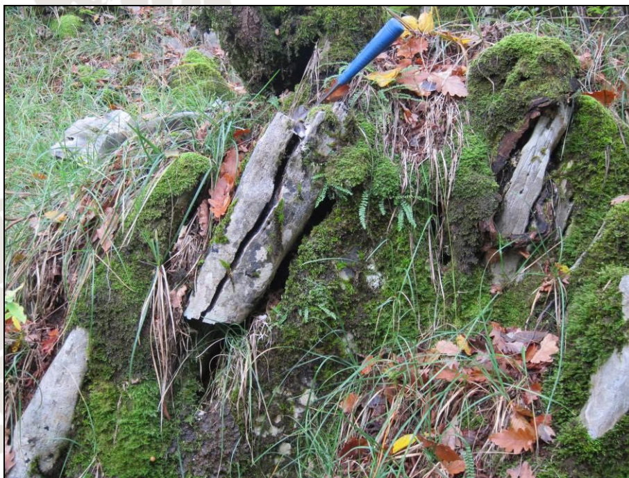
Figure 3.9 A detail from the Gabričje quarry; tectonically related fractures enabled the excavation of limestone plates.
