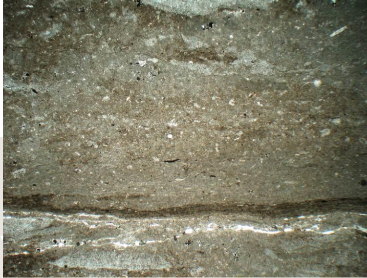
Figure 5.11 Laminated microstructure of Komen PL from the Sežana Fm. usually enable the disintegration of the rock into thinner slabs.
