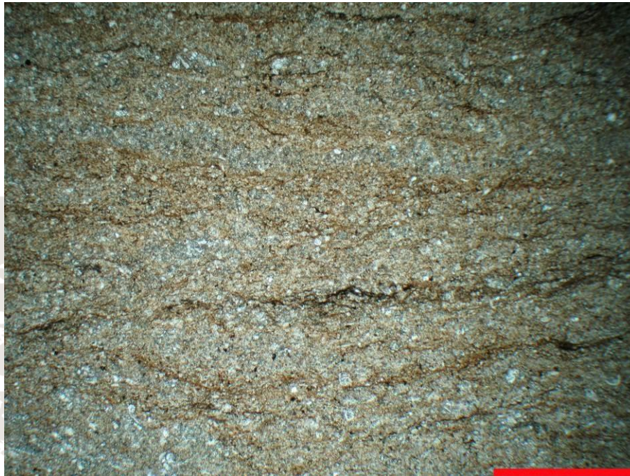
Figure 4.22 A microphotograph of laminated Tomaj limestone. Facies is represented by the thin lamina of skeletal wackestone to packstone and the microcrystalline lamina. The long edge of the photograph is approx. 4mm.
