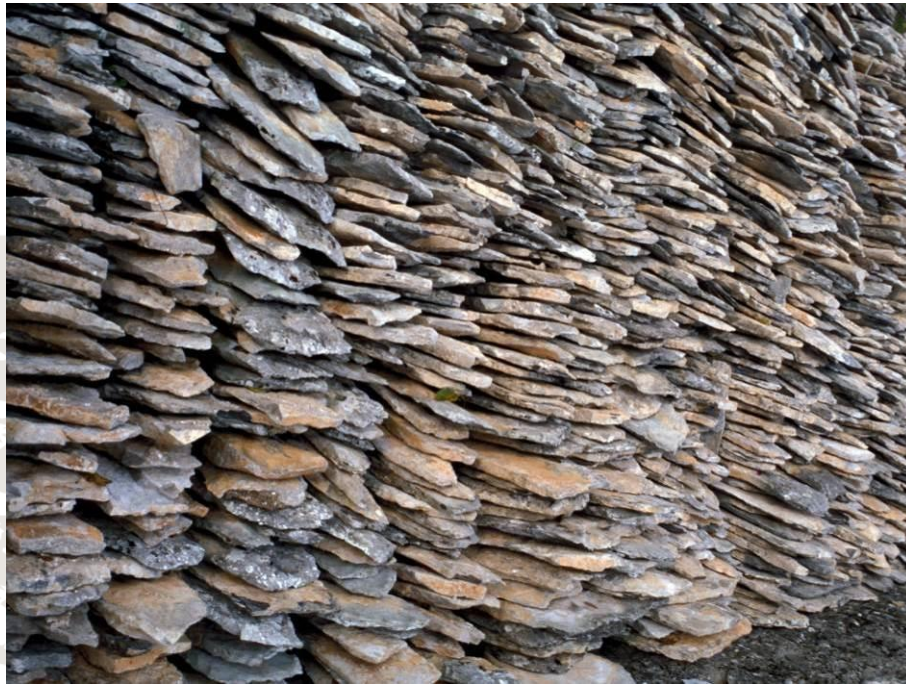
Figure 5.12 Plates of Tomaj limestone ready for roofing (archive photo, B. Jurkovšek).
