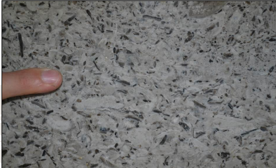
Figure 2.6 The structure of the Kopriva limestone type (easily visible crushed and rounded mollusc shells)
