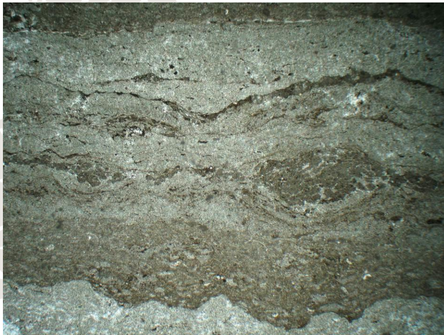
Figure 4.17 A microphotograph of laminated mudstone of Komen limestone from the Sežana Fm. The long edge of the photograph is approx. 5mm.
