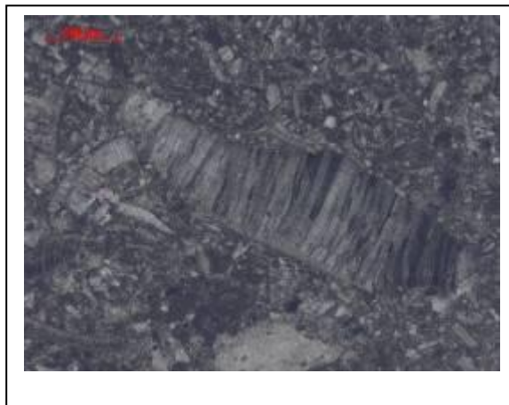
Foto IVB1-4 The bioclasts with prismatic microstructure (crossed Nichols)
