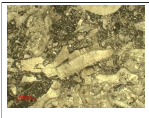
Foto IVB2-1: rudstone with fragments of bivalves, gastropods, brachiopods other bioclasts.
