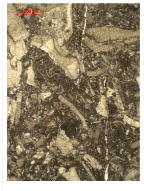
Foto IVC2-4. Fissures exhibiting overstepping architecture.
