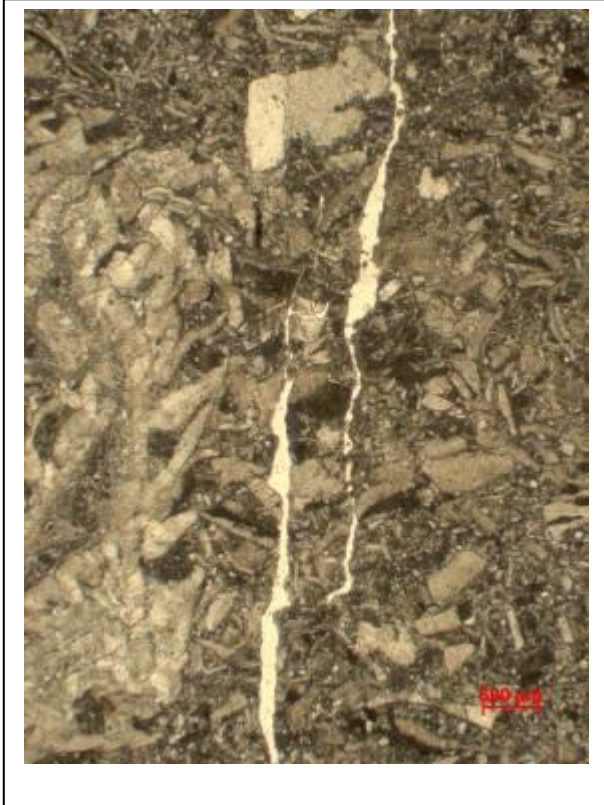
Foto IVC1-3: fissures exhibiting overstepping architecture
