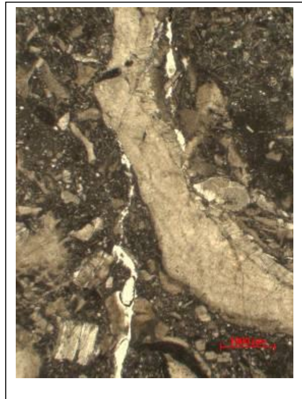
Foto IVC3-2. Termination of fissure at the larger grain.
