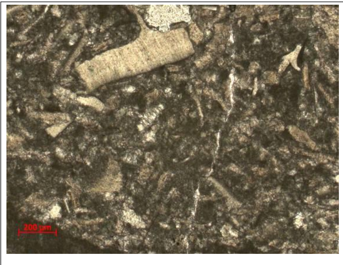
Foto IVB4-9: Partly recrystallised micritic matrix
