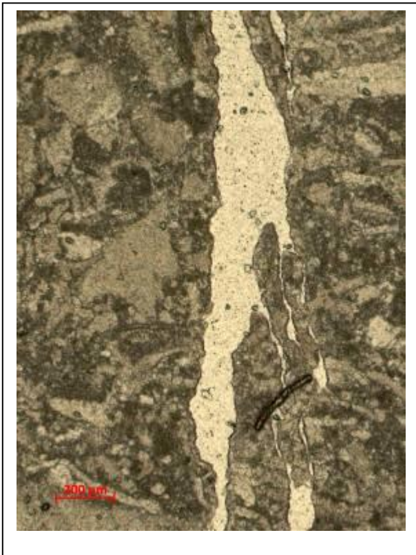
Foto IVC1-5: fissures with straight and smooth walls and slight undulating surface
