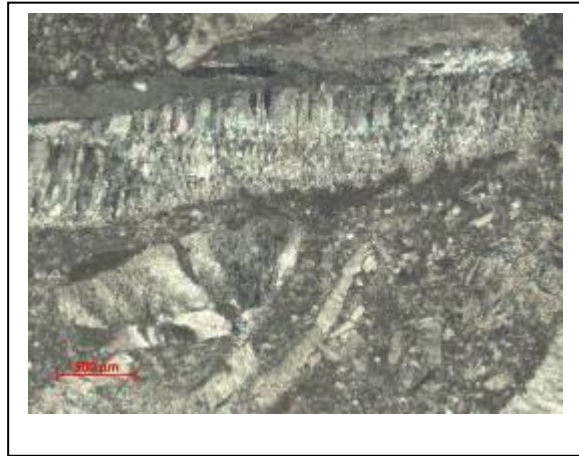
Foto IVB2-4 The bioclasts with prismatic microstructure (crossed Nichols)
