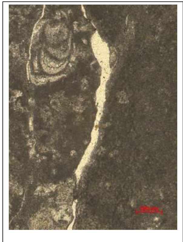
Foto IVC6-10. Fissure with undulating geometry of the fissure wall.
