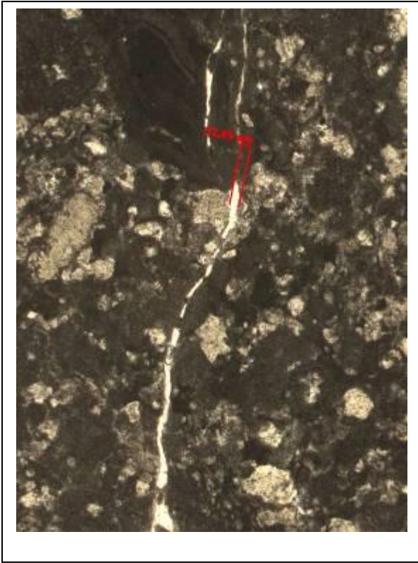
Foto IVC6-7: Small fissures with marked width
