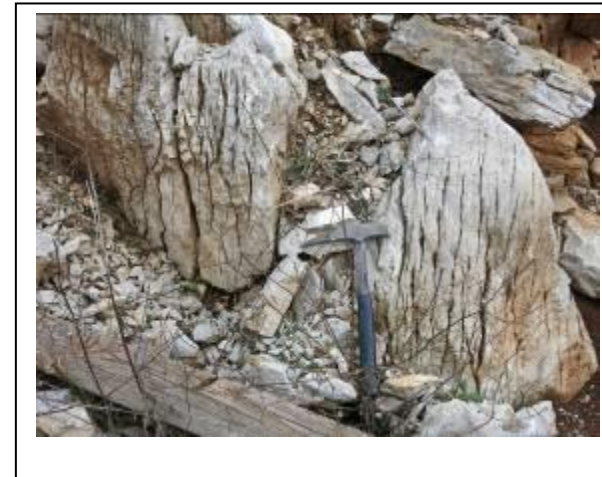
Foto IVA1-3: Fractured limestone of the Debela Griža Quarry
