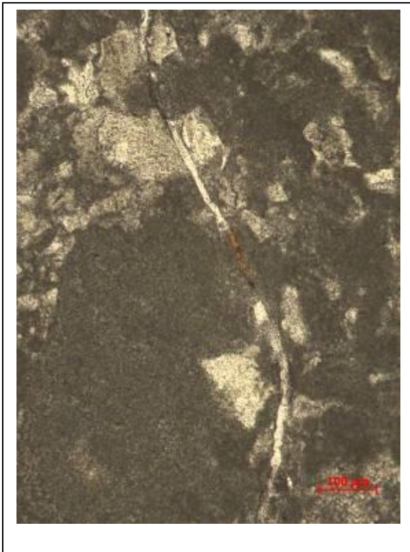
Foto IVC6-11: Clay minerals in the fissure openings.
