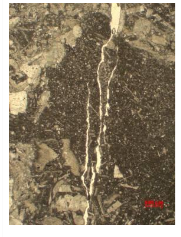
Foto IVC1-4. Main fissure with still attached rock fragments.
