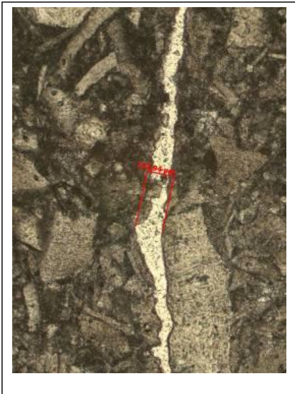
Foto IVC2-3: fissures in grainstone with marked wideness
