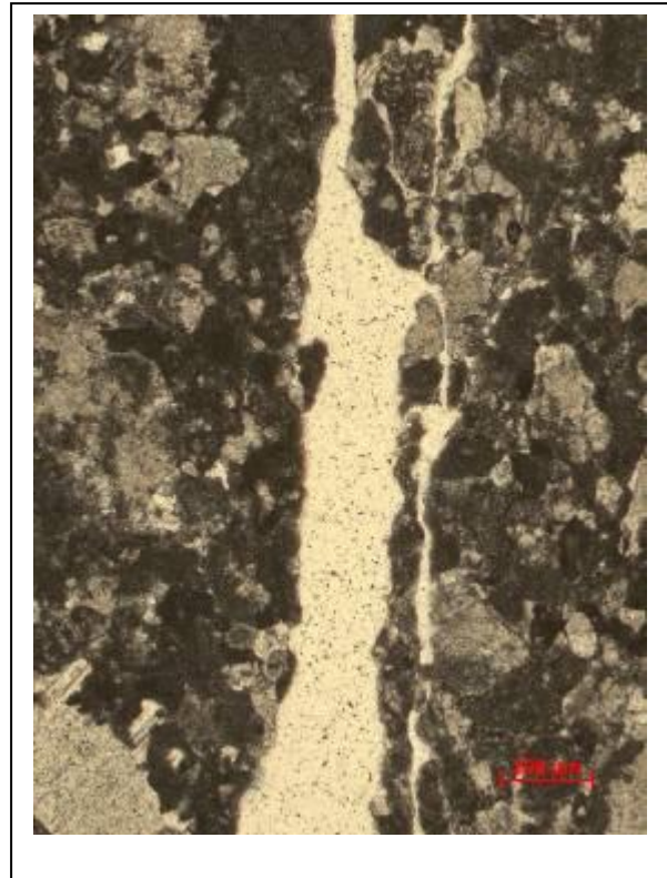
Foto IVC6-4. Smooth walls of the fracture without any sign of recrystallisation.
