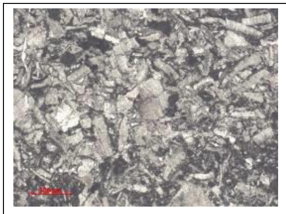
Foto IVB1-1: densely-packed packstone with mainly recrystallised bioclasts ( rudists?).
