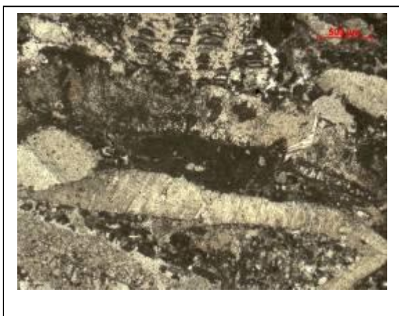
Foto IVB-3: The bivalve bioclasts within the packstone
