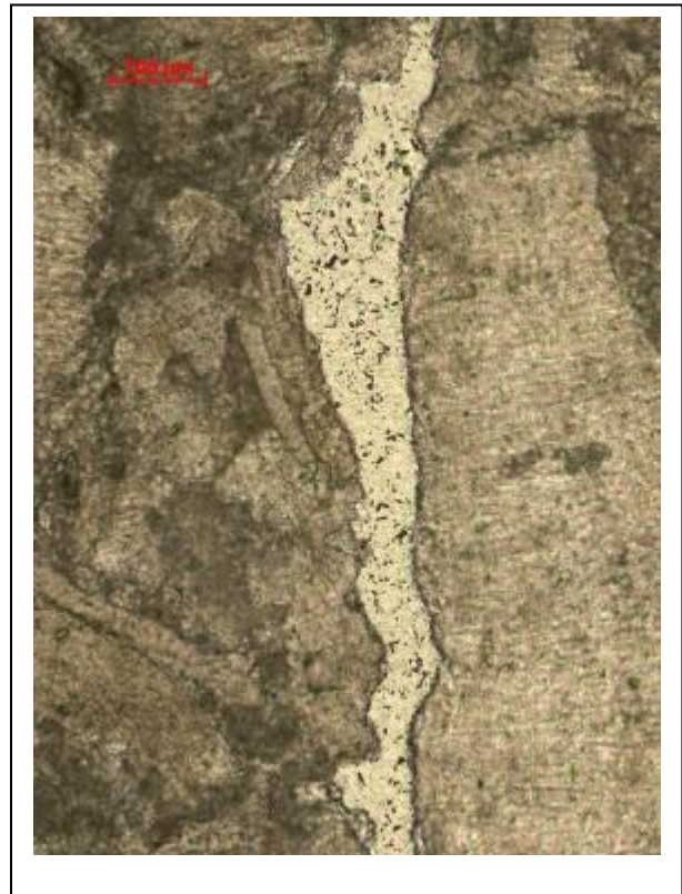
Foto IVC1-6. Small authigenic sparitic-microsparitic grains at the fissure surface.
