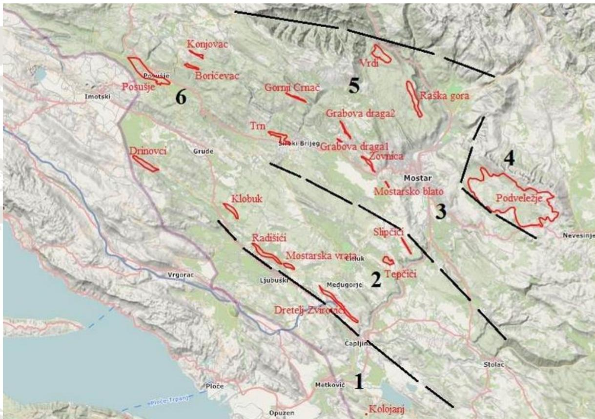
Figure 2.3. Structural-tectonic units in the project area: 1 – Ljubuški-svitava, 2 – Čitluk-Stolac, 3 – Blagaj, 4 – Velež, 5 – Čabulja and 6 – Imotski tectonic unit.
