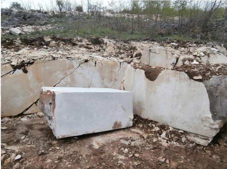
Fig. 2.8. Active quarry of Upper Cretaceous 'Kušanovac' building limestone, in the village of Crno Lokve, near Široki Brijeg.
