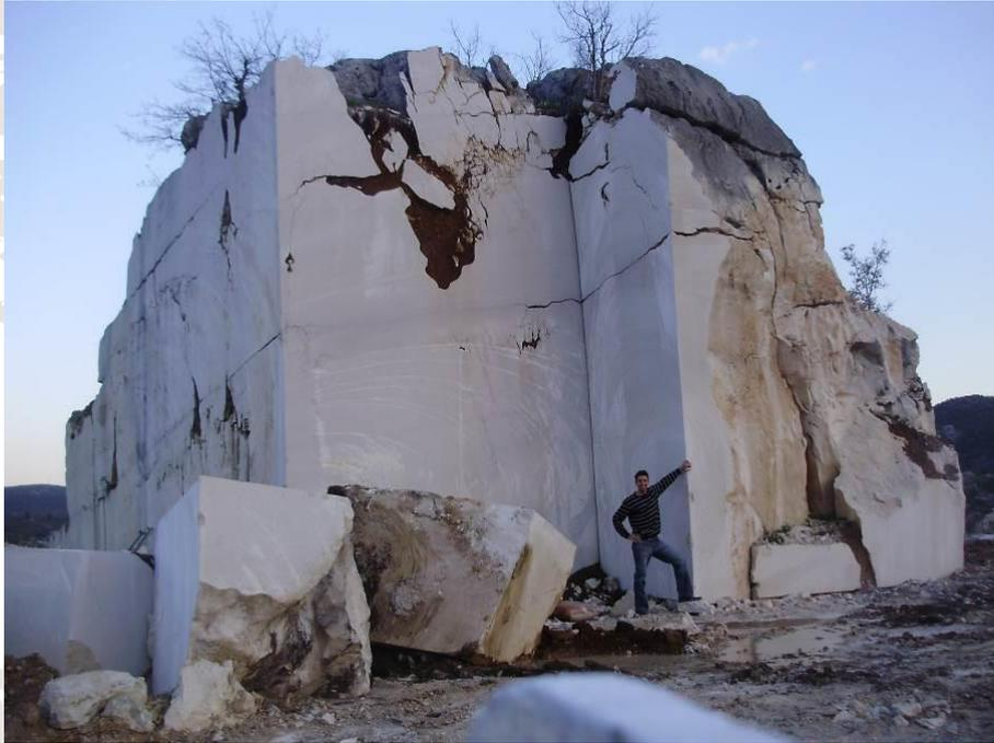
Fig. 2.7. Active quarry of Upper Cretaceous building limestone 'In-Ka-Hercit' in the village of Crveni Grm, near Ljubuški.
