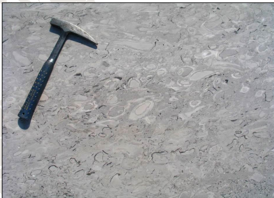
Figure 2.3 The structure of Repen limestone type (easily visible mainly un-fragmented rudist shells)
