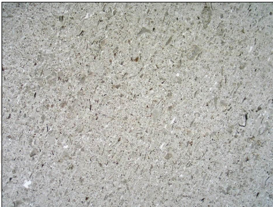
Figure 2.9 The homogeneous structure of Lipica unito limestone type (fine-grained bioclastic limestone)
