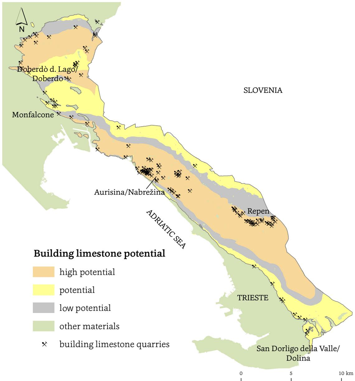
Figure 19: Map showing building limestone potential and locations of the quarries
