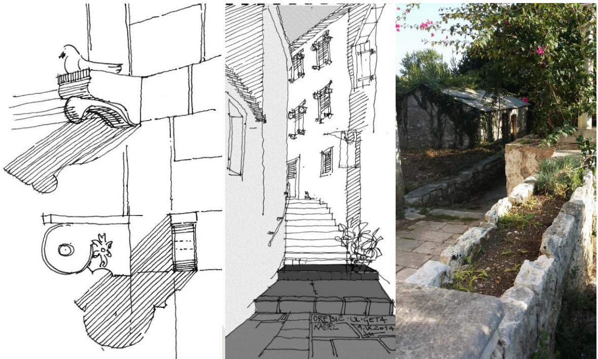
Figure 36: Stone console. Plates may be used as tough for flowers at the top of the border wall. Orebič, Croatia.
