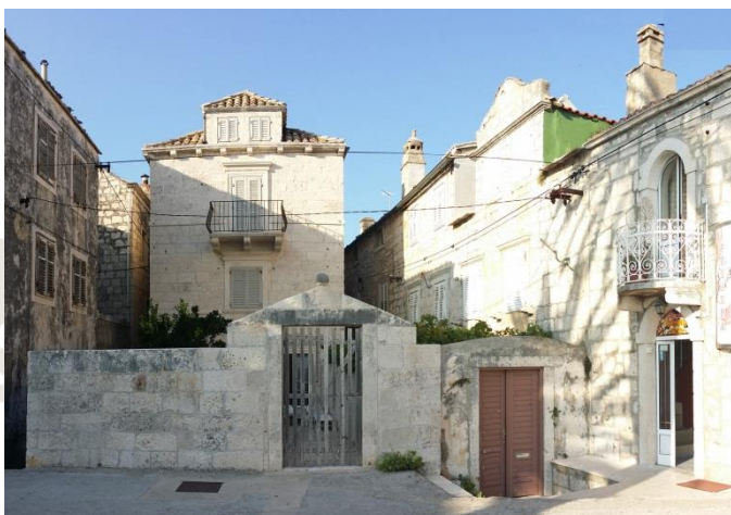
Figure 24: An example of stone houses with vertically set openings. Orebič, Croatia. Foto: Domen Zupančić.
