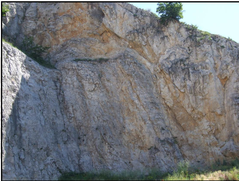
Figure 7. Alveolinid-numulitid limestone in the Scoria quarry above San Giuseppe della Chiusa-Ricmanje unsuitable for stonemasonry due to intense fracturing, despite the bedding in the quarry exhibiting no large displacements.
