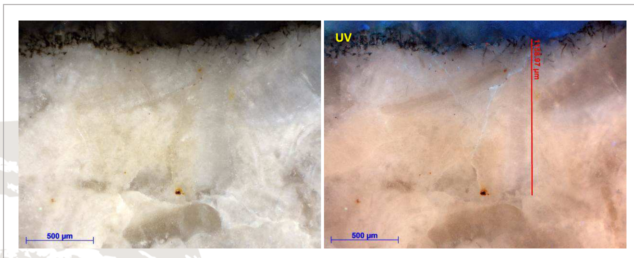
Fractures of the stone structure are visible up to 1 millimeter beneath the exposed surface of the analyzed sample. UV light points out the fractures, where recrystallized carbonate is probably present. Roots of lichen colonies are visible on the sample surface.
