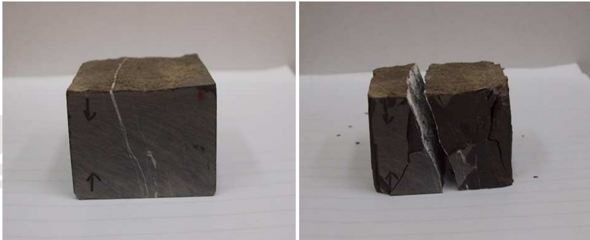
Kazlje sample before and after compressive strength testing.
