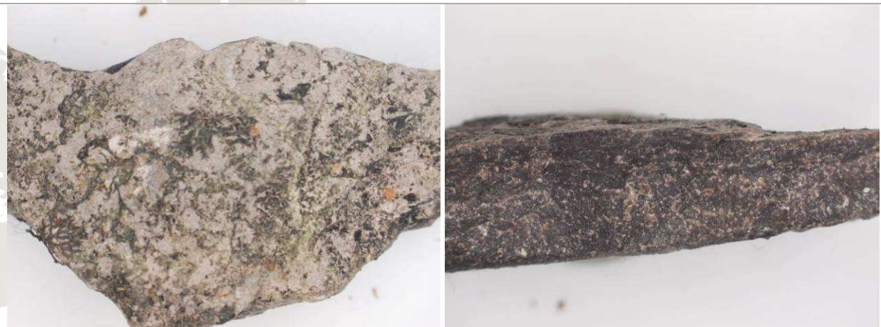
Lichens of various typology are visible on the sample surface. The bulk of the sample has a darker coloration than the surface.
