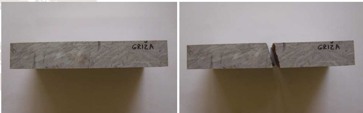
Griza sample before and after flexural strength testing.
